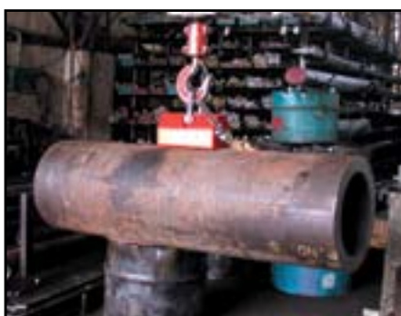
Beveled bottom surface lifts tube steel easily.
