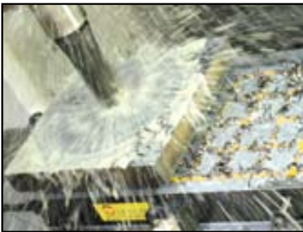
Flood coolant hole-making application
