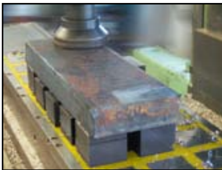
Spring-blocks adjust to hold warped stock
