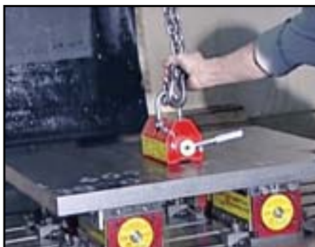
Use to setup CNC machining centers.
