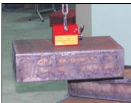
Center magnet on workpiece to lift.
